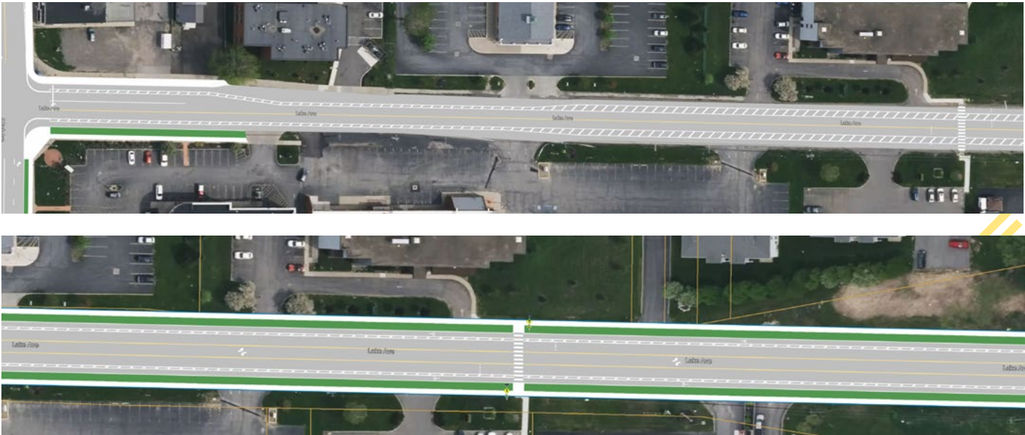
TOP: Quick-build design includes reduced travel lanes with painted hashed buffer zones, a multi-use path in both directions of the road, and a mid-block crossing in front of Our Mother of Good Counsel. BOTTOM: Short-term design with sidewalks, buffered bike lanes, travel lanes, and a two-way center turn lane.
