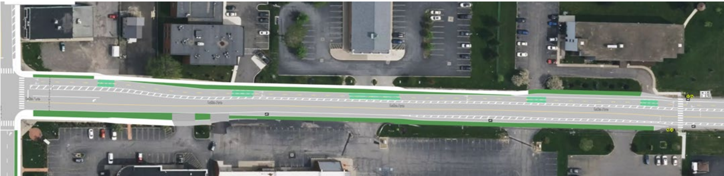
ABOVE: This quick-build design includes reduced travel lanes with a painted protected cycle track on the north side of the road, a multi-use path on the south side, and a mid-block crossing in front of Our Mother of Good Counsel.
